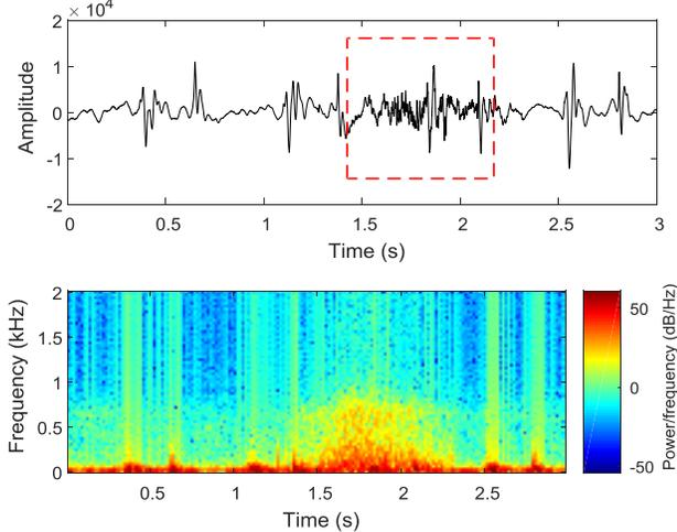
Figure 6. The waveform and spectrum of the data recorded in the second experiment. Upper figure: signal waveform; Lower figure: power spectra obtained by short time Fourier transform (STFT).
