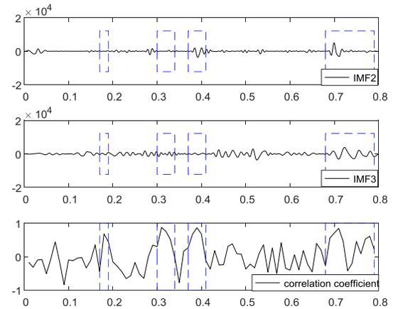
Figure 8. Bandpass filtered  $IMF_2$ ,  $IMF_3$  and their correlation coefficients.
