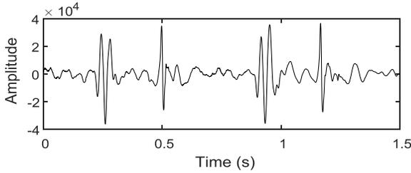
Figure 5. The data after repairing the clipping distortion regions.
