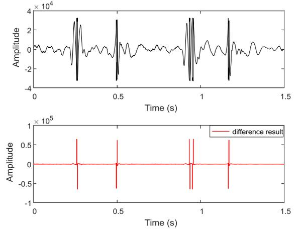
Figure 3. Original signal and its difference result in the first experiment. Upper figure: original signal; Lower figure: difference result.
