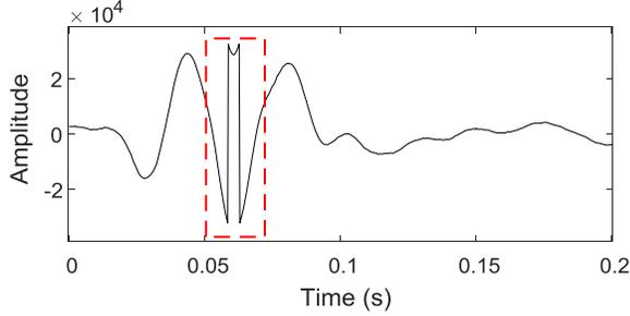
Figure 1. A typical example of clipping distortion, where the red dashed box covers the region where clipping distortion happened.
